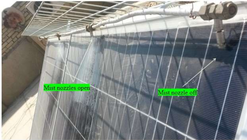
Figure.8 Two nozzles were opened and two nozzles were closed to cool a PV
