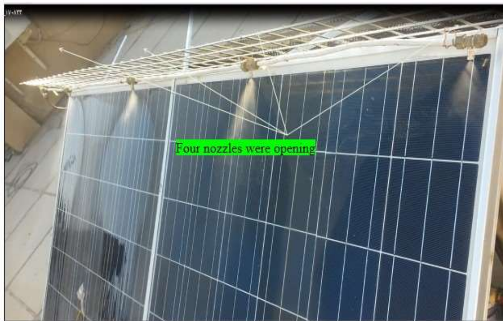
Figure.7 Four nozzles were opening to cool a PV
